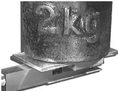
Fig. 4: Linear stage with 10 mm stroke at 2 nm resolution, burdened with 2 kg.
