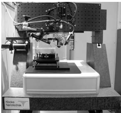
Fig. 14: Micro Production System with small xy-stage ( 100 \times 100 \text{ mm}^2 stroke)
