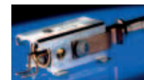
VCSEL-Diode, adhesively bonded after active alignment (Spinner)
